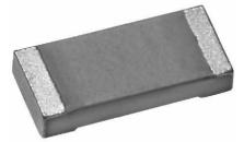
PTS SMD Flat Chip Temperature sensors are the perfect choice for temperature control of electronics operating under varying environmental conditions. The highly controlled platinum thin film manufacturing process guarantees an outstanding stability of temperature characteristics which ensures reliable operation even under harsh conditions. Typical applications include automotive, aviation and industrial electronics.
